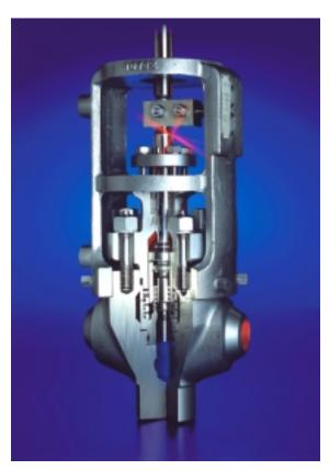
The power station Scholven-Preußen Elektra in Gelsenkirchen has retrofitted four 350 MW power units with 32 GESTRA spray injection valves type ZK. This step has become necessary as the installed valves produced by other manufacturers were difficult to repair and exhibited inadequate tightness values at their characteristic curves.
